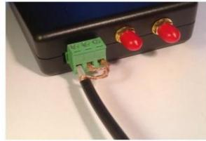
The short length of coax can be terminated with a suitable flying socket (e.g. BNC for use with active loop antennas or SO239 for connection to other existing LF antenna choices.
